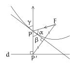
off along the (extension of the) line PP'. And, of course, in reverse: light arriving perpendicular to the directrix will be reflected to the focus.
