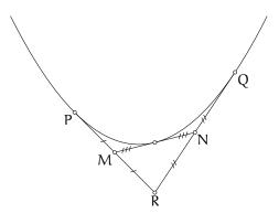
We'll prove this below. For now, just notice how thoroughly routine it is to prove it with modern techniques. Adopting an appropriate coordinate system, the parabola has equation  $y = x^2$ . Let P be the point  $(p, p^2)$ , and let Q be the point  $(q, q^2)$ . Now just compute everything: deploy the techniques of first-year calculus to find the equations of the tangent lines; solve a two-equation linear system to find the coordinates of their intersection; and so on.
